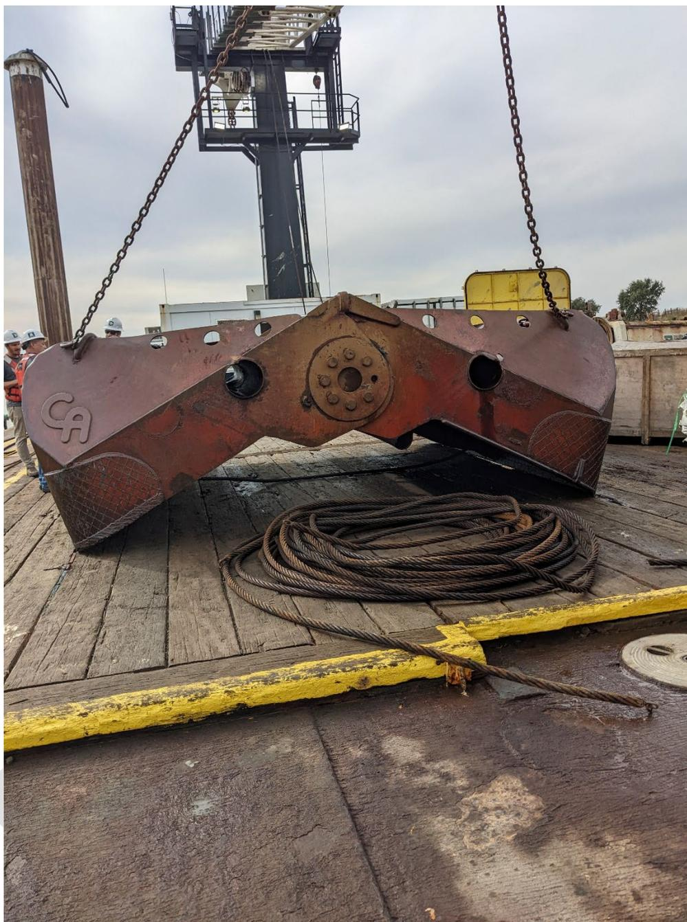
**Figure 4- Closeup of an environmental clamshell dredging bucket. Photo by USACE Sacramento District.**
